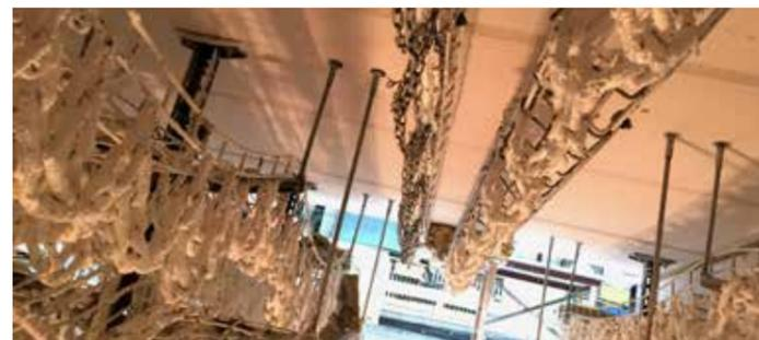
The DIN standard has three approval classes E30, E60, and E90, which correspond to the number of minutes a cable survives a fire. X-Tray has managed all levels and is now E90 certified.
