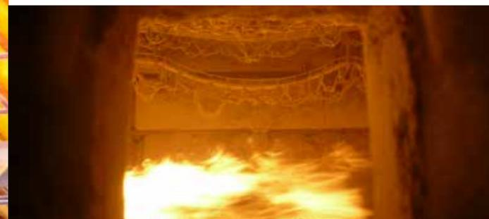
In the bottom of the oven are four large oil burners used to create the fire. The fire rages for 90 minutes, at the end of which the temperature reaches almost 1000° Celsius.
